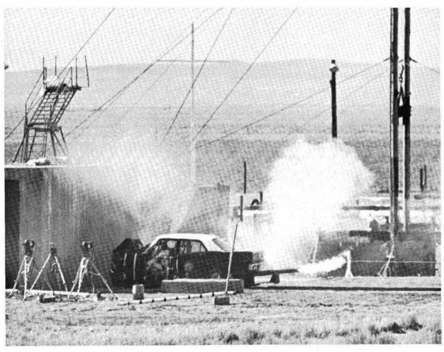
IF YOU'VE WONDERED what happens when your car hits a stone wall at 50mph, then here's the answer. There's the same effect if two cars meet head-on at 25mph. The Area III event is one of a series in which the structural integrity of the type of concrete wall used in a nuclear facility is put to the test. That's a dummy — a real one — in the front seat.
